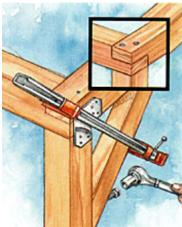
Anchor the six posts to the floor with metal post bases. Use galvanized nails to fasten the bases and posts. Join the beams with half-lap joints (inset). Fasten the braces to the posts and beams with lag screws.
