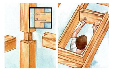
Notch one girt end for the girts to the posts with adhesive and 20d nails (inset).
