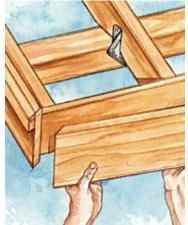
Add the siding to the end Install the subfascia along walls, fastening it to the rafters and timber framing with two facenails at each support.
